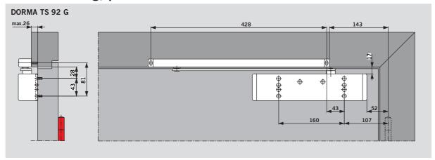
Depending on the structural conditions, the door opening angle with this method of fixing is limited to approx. 120° to 145°. In order to avoid damage to the door or door closer, users are recommended to install a cushioned backstay or a door stop.
