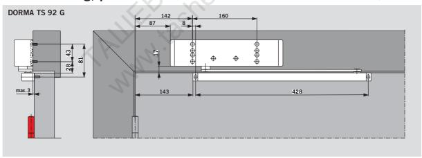
Provided the structural conditions allow, an opening angle of 180° is possible with this method of fixing.
