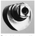
The heart-shaped cam and the linear drive mechanism which characterise all DORMA camaction door closers produce a rapidly decreasing opening torque, so greatly reducing the amount of effort required. This means that even children, the elderly and the disabled can open doors with ease. The user-friendliness of the system is further enhanced by the reliable latching action achieved by the fact that the closing force only rises in the end phase of the cycle.
