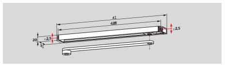
The **DORMA G-N** slide channel assembly comprises the main arm, slide channel, slide block, fixings, screws and end caps. The DORMA G-N slide channel
