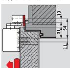
Mounting backplate for G-N For fixing the slide channel to the door frame where there is no means of direct mounting.
